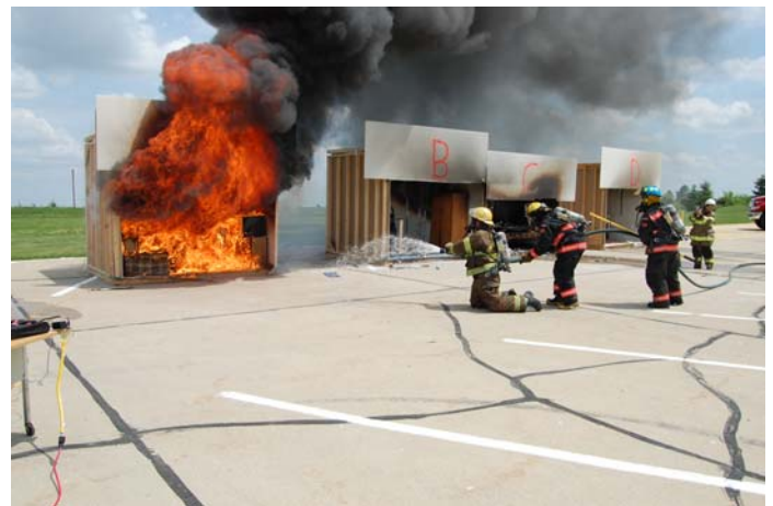
Above and Below: The first cell was a living room and the fire in this room was incendiary with a flammable liquid being applied to a couch with foam cushions. Above sprinkler. Below no sprinkler
