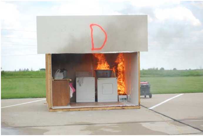
Above: The last cell was a laundry room scenario with a simulated dryer fire from lint build up being the cause.
