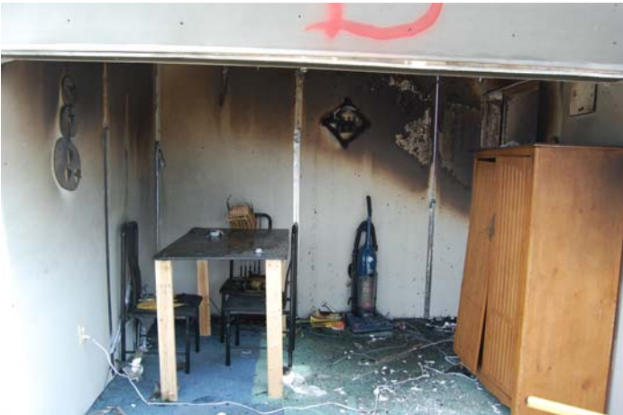
Above and Below: The second cell was a double cell with two of the 8x10 cells being placed together and a doorway placed in the common wall the cells shared.
