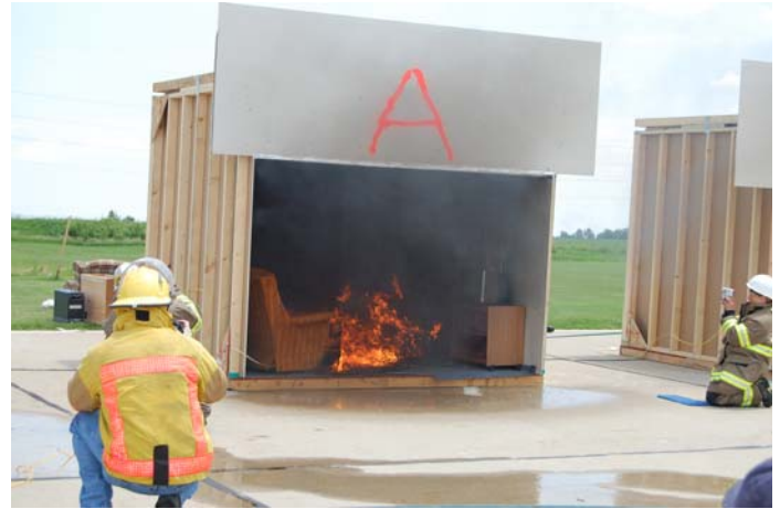
Above and Below: The first cell was a living room and the fire in this room was incendiary with a flammable liquid being applied to a couch with foam cushions. Above sprinkler. Below no sprinkler
