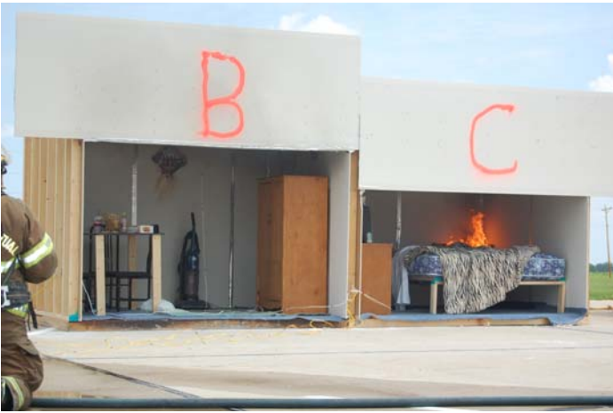
Above and Below: The second cell was a double cell with two of the 8x10 cells being placed together and a doorway placed in the common wall the cells shared.
